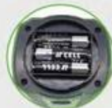
3AA batteries for backup
